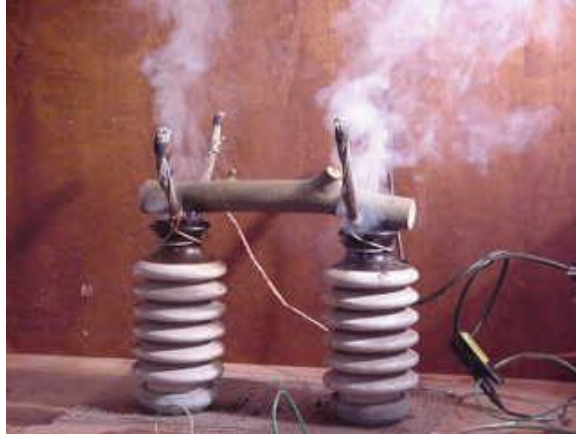
Figure 1. Specimen under high voltage testing.
